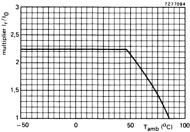
Fig. 4 Typical ripple current as a function of ambient temperature; I_0 = ripple current at 85 °C and 100 Hz.
